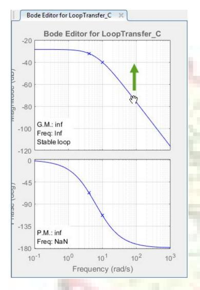
Drag the magnitude response upward until the crossover frequency is about 3 rad/s.
